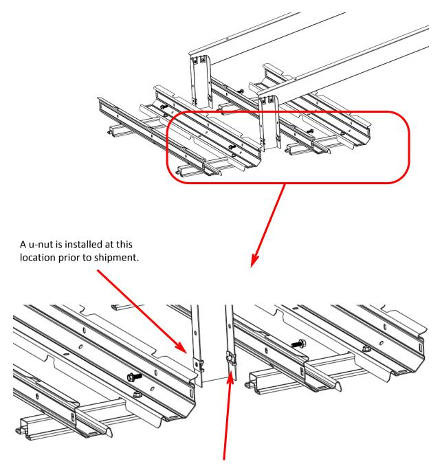
The additional u-nuts supplied with the shipment must be installed at this location on the front vertical legs of the support rail assemblies
