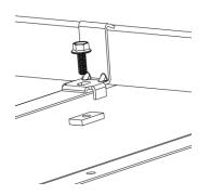
One (1) module clamp installed with one (1) M6x1 bolt and one (1) rectangular nut.
