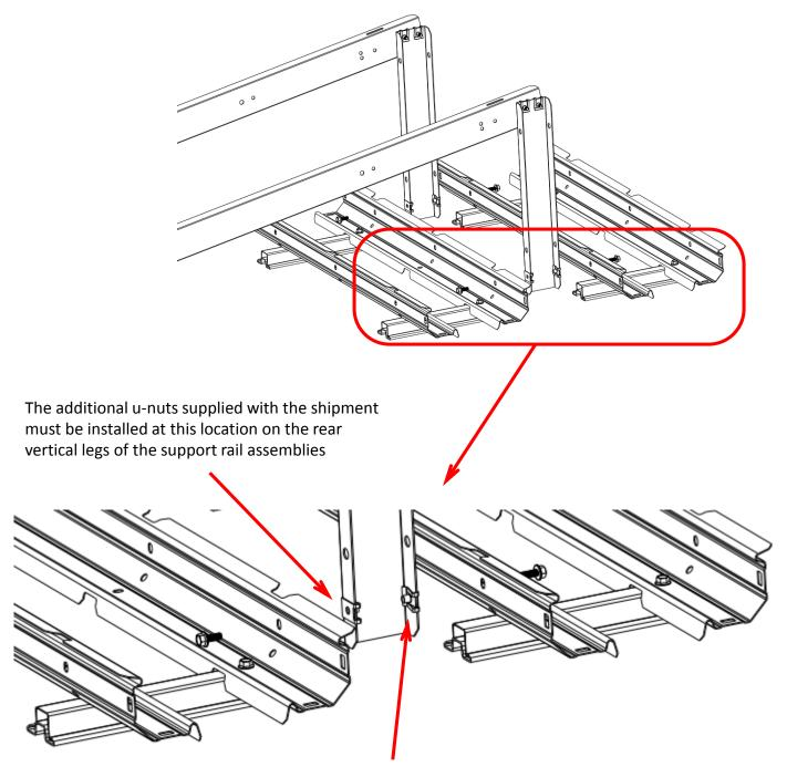
A u-nut is installed at this location prior to shipment.
