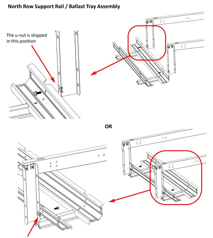
The u-nut must be moved to this position when tucking the ballast tray under the support rail.
