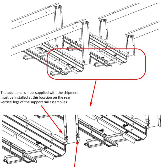
A u-nut is installed at this location prior to shipment.
